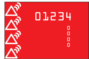
System fault alarm (red). The numbers relate to the error that caused the system fault.
