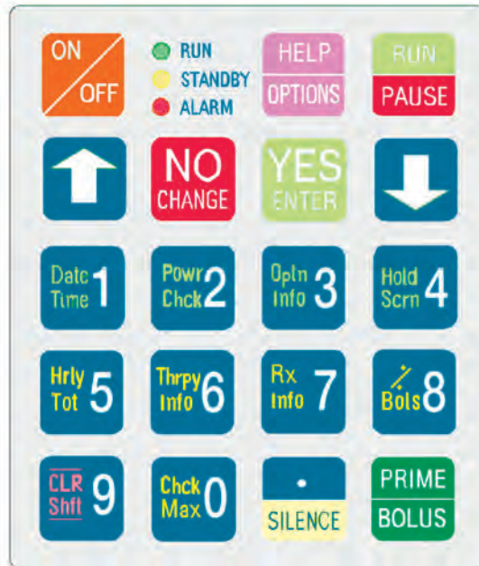
Figure 2.2 IOD Keypad with Info-On-Demand Feature
