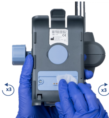
Figure 11.1. Cleaning Electric Connectors
