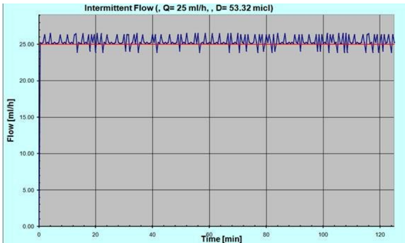
Figure 12.4. Delivery Startup Graph, First 2 Hours of Test Period, 25 mL/h
