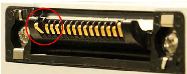
Bent pin on a male IUI connector
