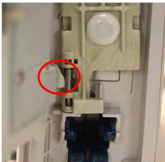
Broken platen lower hinge bracket
