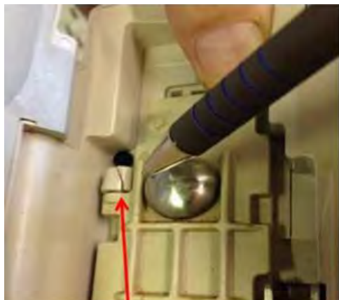
Cracked hinge on membrane frame
