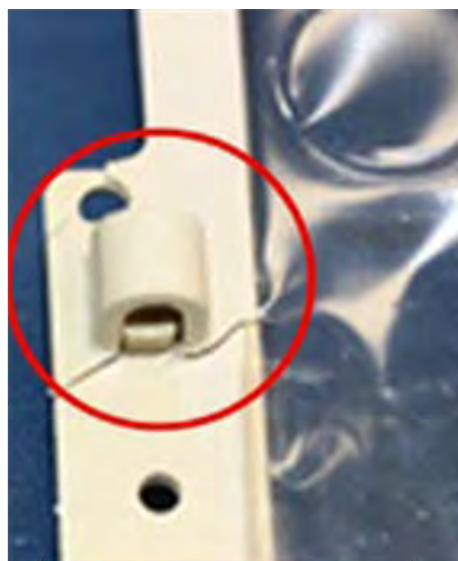
Membrane frame breakage
