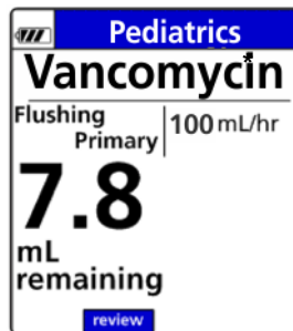
Figure 110. Primary Line Flush Status Screen.
