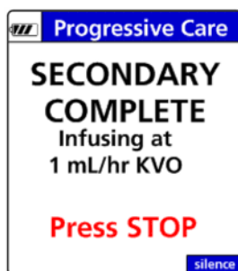
Figure 59. Secondary Complete: KVO Alarm.
