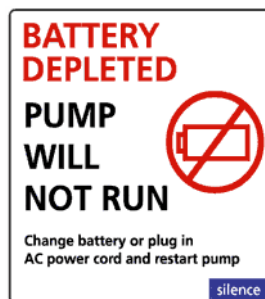
Figure 138. Battery Depleted Alarm.
