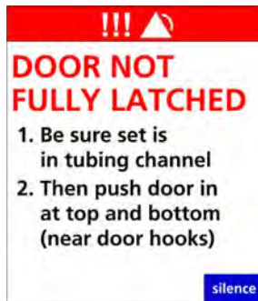
Figure 9-11. Door Not Fully Latched
