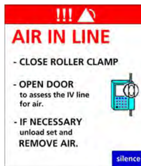
Figure 9-4. Air in line Alarm
