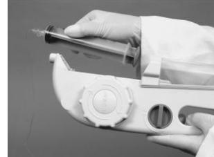
After the infusion is complete, turn the pump OFF and wind the large knob clockwise until the black tab is at the end of its track. Remove the empty syringe by gently pushing it back and up out of the pump.
